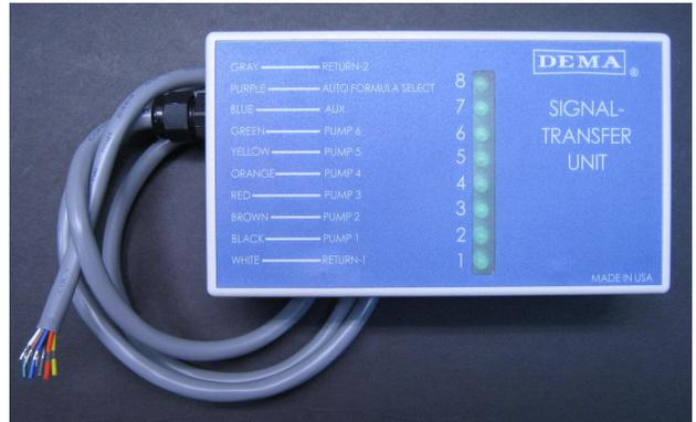
The wiring of the DEMA STU-II is shown on the front label. The supply signals from the laundry machine can be 12VAC-250VAC. There are 2 common wires (white and gray). The out of the box product from DEMA can use either one or both commons. It is not necessary to wire both commons. However, both commons can be wired to the machine common or return. All trigger wires and commons are in a jacketed cable assembly.
