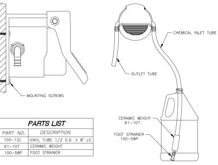
**SERVICING:** Flush with warm 4. water to dissolve any dried fluid.
