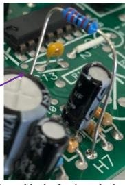
To enable the 3-minute lockout cut **ONE** leg of the **HIGH** resistor located in H6 &
