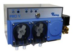
**Pro V** Detergent, Rinse, & Sanitizer Warewash Control System **The Viking Pro V\*** is a 3 product, liquid rinse, liquid sanitizer & (liquid or powdered / solid) detergent probe controlled warewash dispenser for high temp dish machines. The Pro 5 can be ordered with 2 internal transformers, 2 internal transformers and a pressure switch, or as an external transformer unit.
